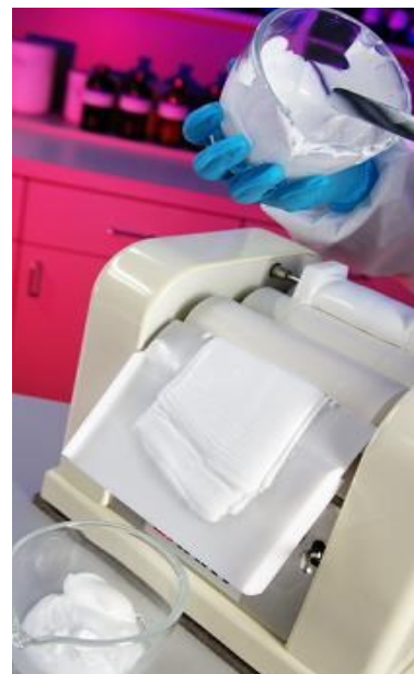
Ointment Mill used to homogenize and “mill down” active drugs into our pain relieving “SHINGLES” cream
